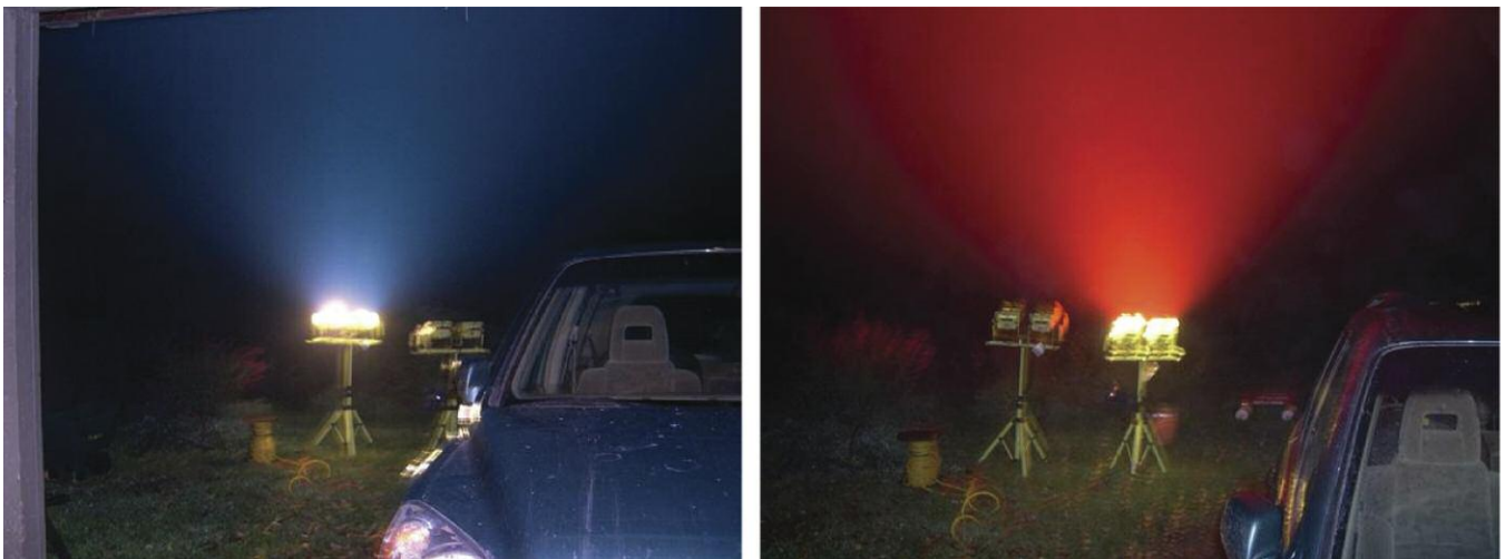
Figure 1. 1500W halogen test lights with blue and red filters used to study the impact of light upon migrating birds.
